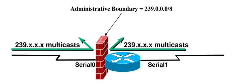
• Configured using the 'ip multicast boundary <acl>' interface command
