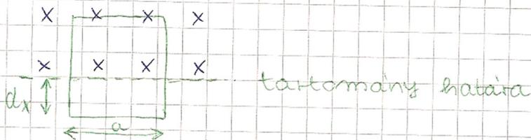
$\mathcal{U} = - \frac{\partial \phi}{\partial t} = - \frac{\partial}{\partial t} (B \cdot A) = -B \frac{\partial A}{\partial t} = -B \cdot a \frac{dx}{\partial t} = -B a v$
