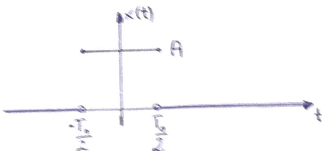
$$\begin{aligned} X(j\omega) &= \tilde{F}\{x(t)\} = \int_{-\infty}^{\infty} x(t) e^{-j\omega t} dt = A \int_{-T_0/2}^{T_0/2} e^{-j\omega t} dt = A \left[ \frac{e^{-j\omega t}}{-j\omega} \right]_{-T_0/2}^{T_0/2} = \\ &= A \left( \frac{e^{-j\omega \frac{T_0}{2}} - e^{j\omega \frac{T_0}{2}}}{-j\omega} \right) = 2 \frac{T_0}{2} A \frac{e^{j\omega \frac{T_0}{2}} - e^{-j\omega \frac{T_0}{2}}}{2j\omega \frac{T_0}{2}} = T_0 A \frac{\sin(\omega \frac{T_0}{2})}{\omega \frac{T_0}{2}} \end{aligned}$$
