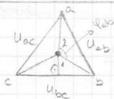
$$\begin{aligned} \left( \frac{U_{bc}}{2} \right)^2 + \left( \frac{3}{2} U_a \right)^2 &= U_{ab}^2 \Rightarrow U_a = 61,1010 \cdot e^{j0^\circ} [V] \\ \left( \frac{U_{bc}}{2} \right)^2 + \left( \frac{1}{2} U_a \right)^2 &= U_b^2 \Rightarrow U_b = 50,3322 \cdot e^{j127,37^\circ} [V] \\ U_c &= 50,3322 \cdot e^{j127,37^\circ} [V] \end{aligned}$$
