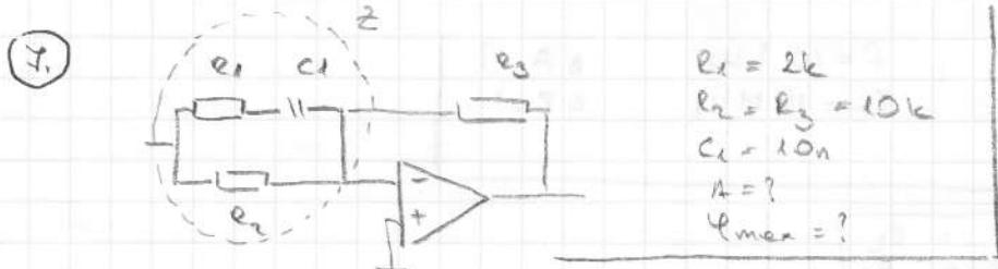
$$A = - \frac{R_2}{R_1} \Rightarrow A = \frac{-R_3}{Z} = \frac{-R_3}{Z_1 \times R_2} = \frac{-R_3}{(\frac{1}{j\omega C_1} + R_1) \times R_2}$$
