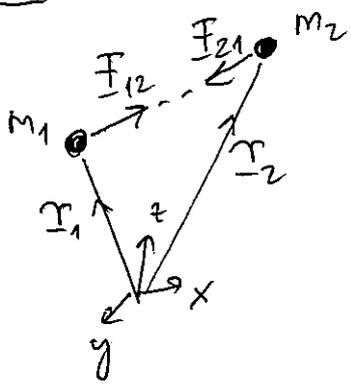
$$F_{12} = -\gamma \cdot \frac{m_1 m_2}{|r_1 - r_2|^3} \cdot (r_1 - r_2)$$
