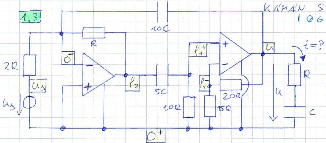
$$\left. \begin{array}{l} l_1^-: 0 = \frac{l_1 - u}{20R} + \frac{l_1}{15R} \\ l_1^+: 0 = \frac{l_1}{10R} + (l_1 - l_2) \cdot j\omega 5C \\ 0^-: 0 = -\frac{u_s}{2R} - u j\omega 10C - \frac{l_2}{R} \\ y: i = \frac{u}{R + \frac{1}{j\omega C}} \end{array} \right\}$$
