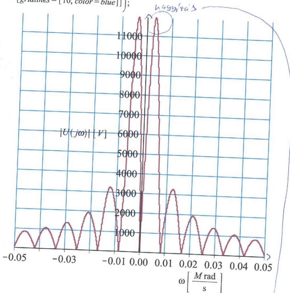
>  $\text{plot}\left(\text{abs}(u), \omega = 0.0034 .. 0.0035, \text{numpoints} = 10000, \text{labels} = [\omega \left[ \frac{\text{Mrad}}{\text{s}} \right], |U(j\omega)| [\text{V}]], \text{axis} = [\text{gridlines} = [10, \text{color} = \text{blue}]]\right);$
